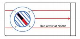
Around the needle is a moveable 'housing'. This has the letters N, S, E, W marked on it to indicate the directions north, south, east and west. Some compasses also show the intermediate directions: northeast, northwest, southeast and southwest.
